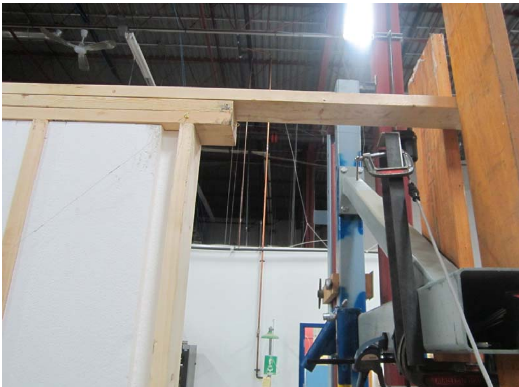
Photo 2. Guides installed to prevent twisting of test wall assembly during testing
