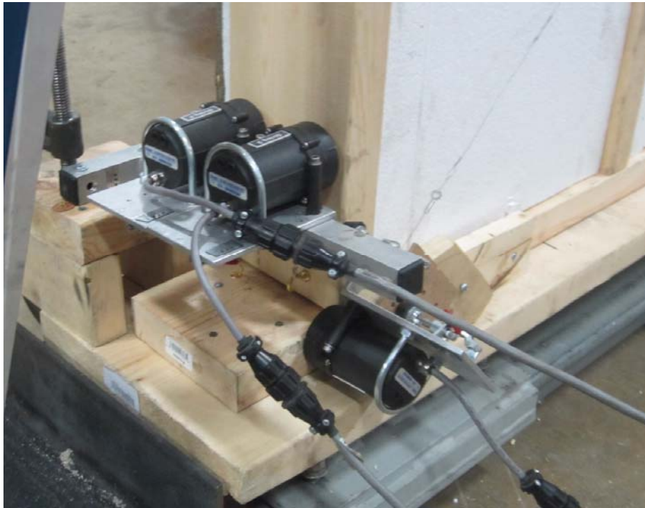
Photo 3. String Potentiometers for measuring deflections installed at bottom corner of test assembly
