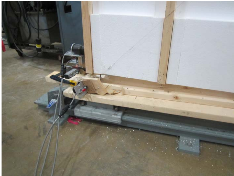
Photo 4. Ultimate failure of shear wall at the end of the test. Vertical stud uplifted from the sole plate.
